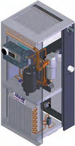
*AHT series includes an aftercooler, a pre-filter and a dryer in a single unit; and it is the modern evolution of a product already introduced in the market from Friulair, but update with latest technologies. This dryer combines of a copper tube and aluminium fin air cooled aftercooler, a pre-filter with automatic drain and the established **Alu-Dry Module Refrigerant Dryer**, a completely aluminium heat exchanger built to a Friulair patented design. The product has numerous advantages :*
